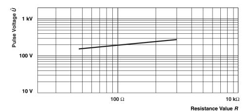
Pulse load rating in accordance with IEC 60115-1, 4.27; 1,2  $\mu$ s/50  $\mu$ s; 5 pulses at 12 s intervals; **1.2/50 Pulse** for permissible resistance change 0.5 %
