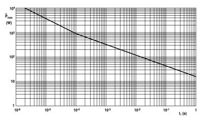
Pulse on a regular basis; maximum permissible peak pulse power  $\mathbf{\hat{P}}_{max}$  as a function of pulse duration  $(t_i)$  for single pulse condition
