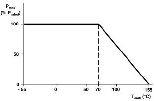
The power that the resistor can dissipate depends on the operating temperature
